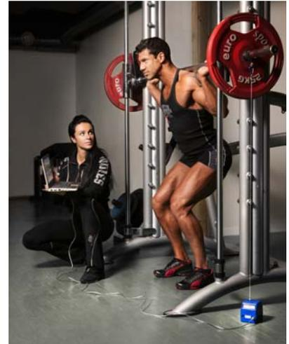
For use with weights, its nylon wire is hooked to the weight stack, barbell or dumbbell and measures the lifting speed during exercise, which is then used to compute power and other variables in the software.
